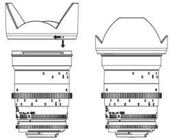
Align the attachment reference point on the hood with the hood reference point on the lens, push the hood onto the lens and turn the hood clockwise until it makes a clicking sound.
