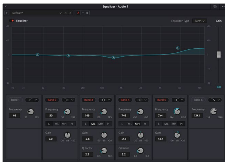
The 6 Band parametric equalizer that can be applied to every track
